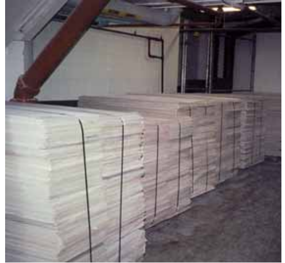
Pallets of old, discarded ceiling tiles at Sun Life Plaza await pick-up by Armstrong, which will use them in the manufacture of new acoustical ceilings.
