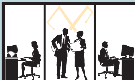
Traditional Closed Office: Sound is repeatedly reflected off all surfaces and absorbed at the ceiling with NRC 0.55 minimum – but these standard ceilings are unacceptable for effective open plan design/call centres.
